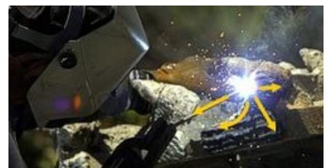
metal becomes hot (the orange-red glow) by the transfer of heat from an arc.
